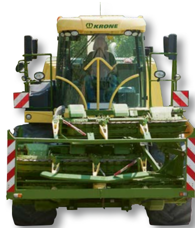
Compact transport width: the three-section EasyCollect
